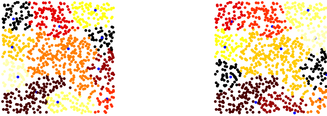
Figure 8: Example of clusters organization for 1000 nodes with a radius R = 0.1 with the degree heuristic (a) and with 1-density heuristic (b).
